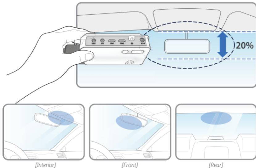
**TIP:** The adhesive is extremely sticky. Avoid touching the adhesive to the windshield until the mount is properly positioned and aligned.
