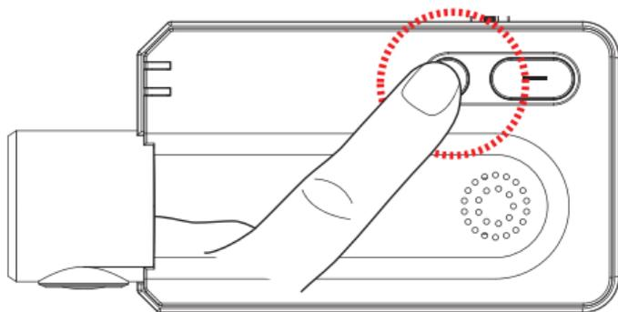
**!** In case of turn the system off by holding the power button, you have to press and hold the power button again in order to restart the system.
