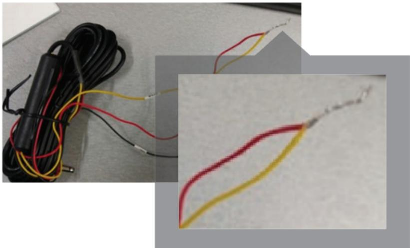
Twisted cable should connect to power supply of fuse which is operated.
